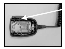
The correct PTT lever will be identifiable at any time by the letter 'B' marked inside the PTT lever.
